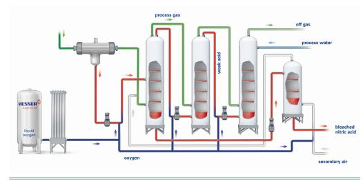
Figure 1. Flow chart of nitric acid production with different introduction points.
