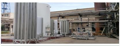
Figure 4. Test equipment including a mobile tank, vaporisers, fundaments, regulation skid and flexible hoses.
