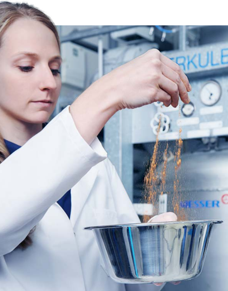
Cold grinding ensures that the material being ground does not coalesce and agglutinate. Spices retain their flavours.
