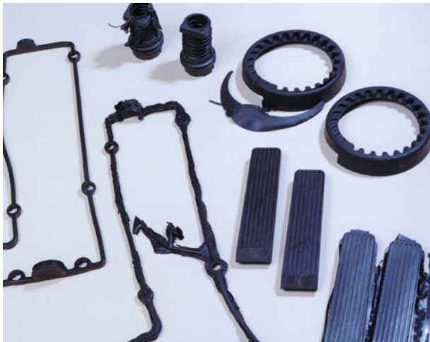
Rubber parts before and after deflashing
